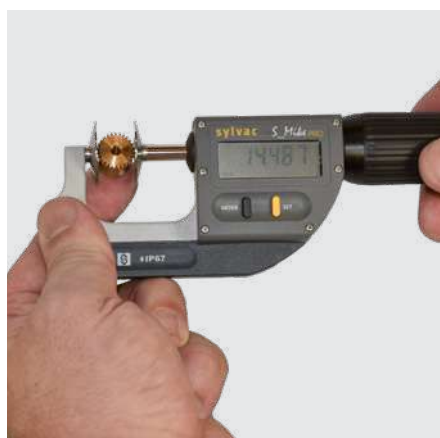
Part measurement with a S_Mike PRO Disk
