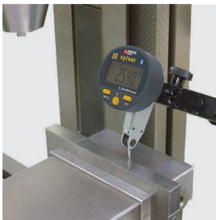
Checking the alignment on milling machine.
