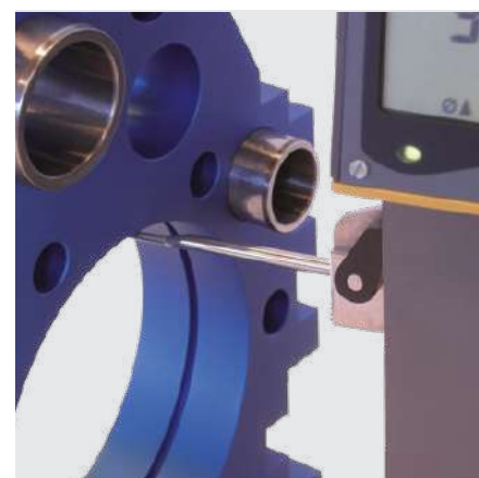
Internal measurement with ruby ball probe Ø 3 mm, 930-2101 (standard)
