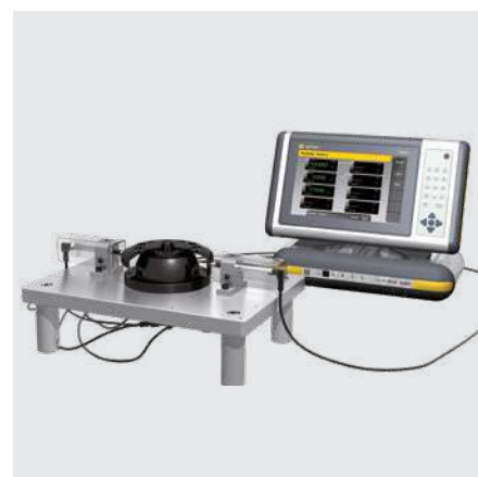
Capacitive probes on a jig
