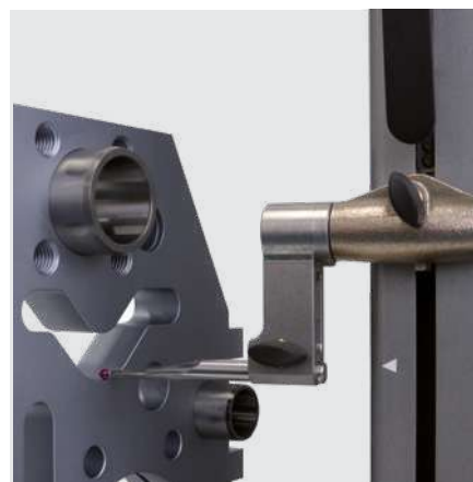
The motorisation guarantees a perfectly constant measuring force
