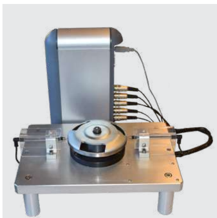
Capacitive probes connected to a D200S.
