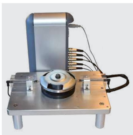
Capacitive probes connected to a D200S
