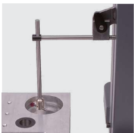
Internal groove measurement with accessories 930-2108, 930-2110 and 905-2207
