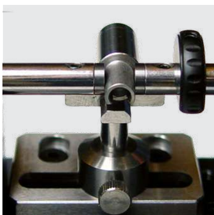
External measurement with anvils Ø 6.5 and XYZ table
