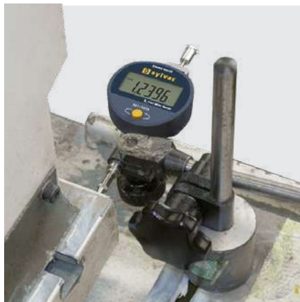
Measurment of the vertical displacement of an element
