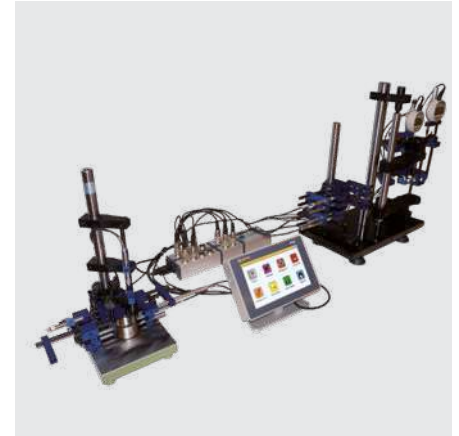
Probes and indicators connection through M-BUS inputs
