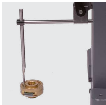
Depth measurement with accessories 930-2108 and 930-2105
