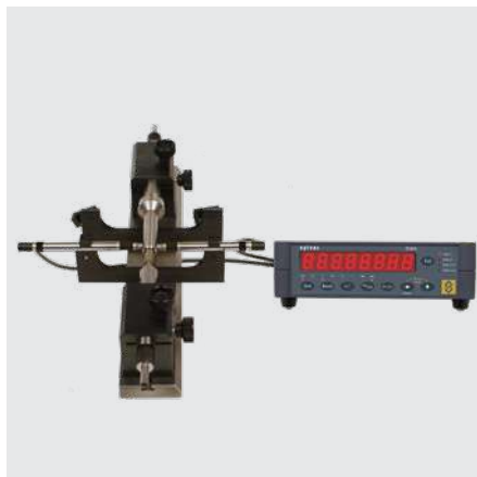
Measuring a shaft with 2 probes (A+B)
