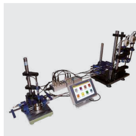
Probes and indicators connection through M-BUS inputs
